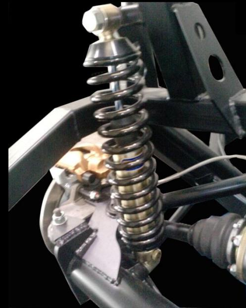
***“GAZ gas-filled coil-over damper assemblies with full adjustment for height and damping”.***
