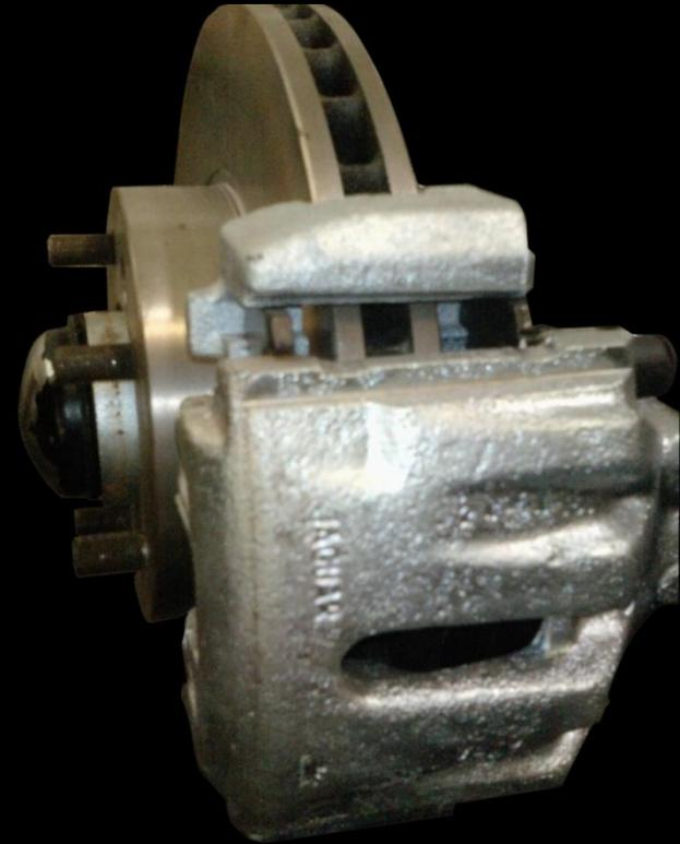
***“Handbrake function provided by centre, drum & shoe section, of each rear disc”.***
